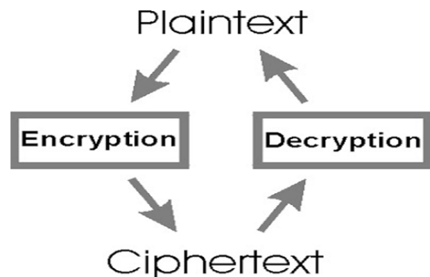
Figure 1: Conversion of plain text to cipher text and vice versa
